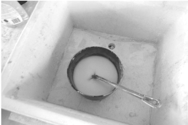
18 The plaster is settling in the water and all the air bubbles have risen.
