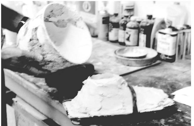
19 The plaster is being poured into the negative cast.
