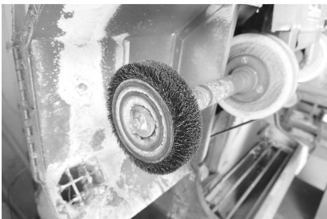
14 Cleaning and shaping tools. Wire brush on Sutton sanding machine.
