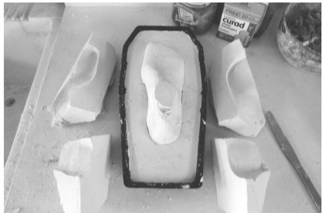
21 The top of negative cast has been separated. The inner cast (which is a cast of a last) is ready to be removed.
