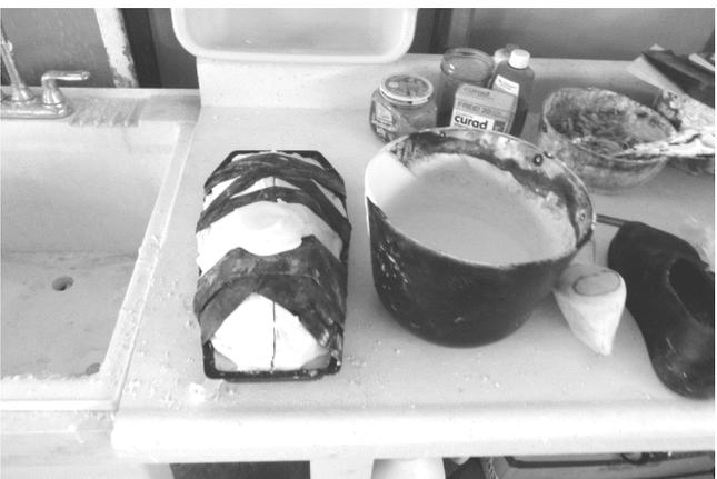
20 The negative cast is full of plaster. It needs to dry a couple of hours.
