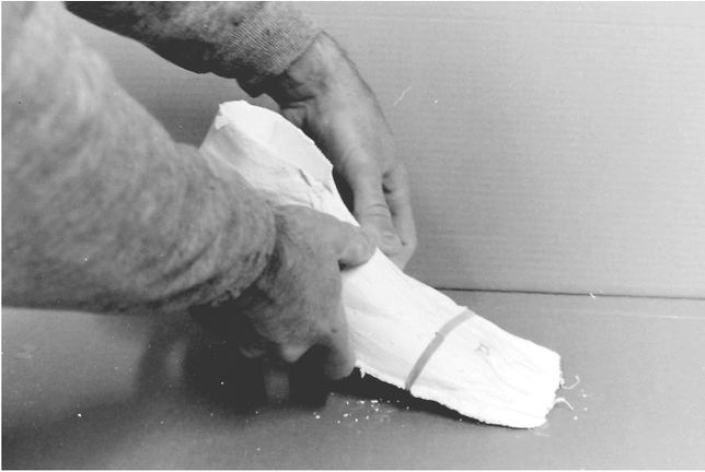
5 The shell is tilted and shook so there are no air bubbles in the plaster.
