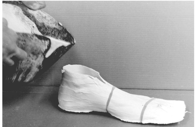
2 The plaster is fluffed and put in the bowl. Enough water is added to cover the plaster and let all the air escape. After the bubbles have risen and excess water is poured off, the plaster is stirred to uniform liquid consistency.
