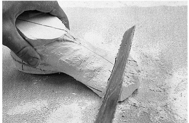
16 An angled vertical cut is made down to the horizontal cut.
