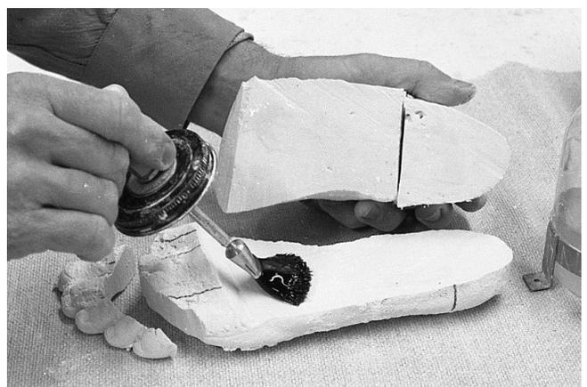
36 Applying glue to the bottom.
