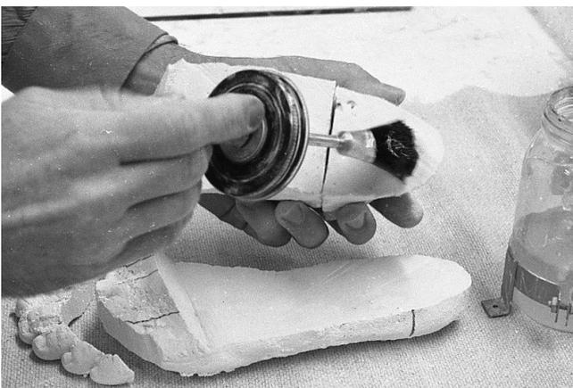
35 Ditto. Plaster parts can be bonded together with high solids latex (undiluted). The latex bonding will take longer to cure.
