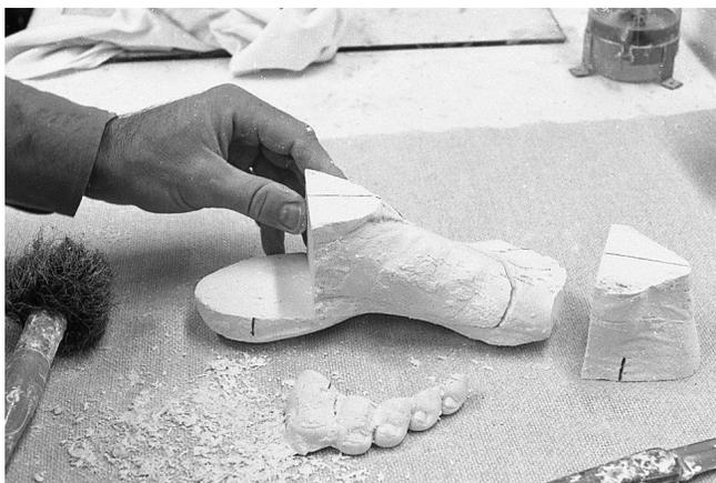
29 The top front of cast is put onto the bottom.
