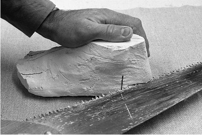
13 A horizontal cut is made with a drywall (plaster) saw.
