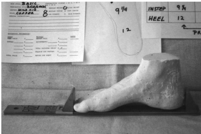
11 The Ritz® stick can help with the measuring of the length of the foot.
