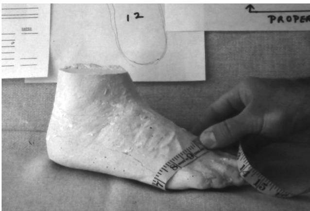
7 Lateral view of measuring the ball of the foot.
