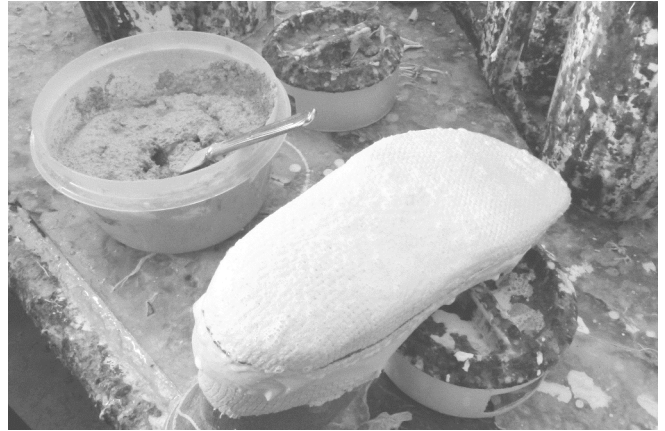
24 A uniformly wet "mud" is desired. It should be soft and self standing with very little slump. That is the desired consistency for the mix. It should spread easily when applied.
