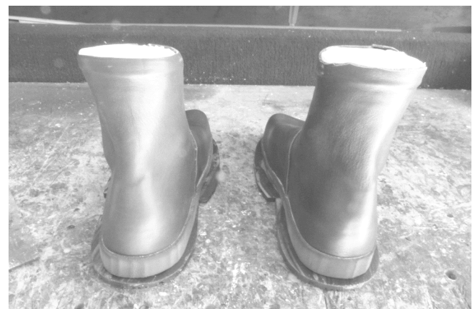
106 The outer soles have been glued and attached to the boots. Notice the oversize sole was cut in the middle to make it match the length of the boot. This is sometimes necessary when making footwear for wide and/or short feet.
