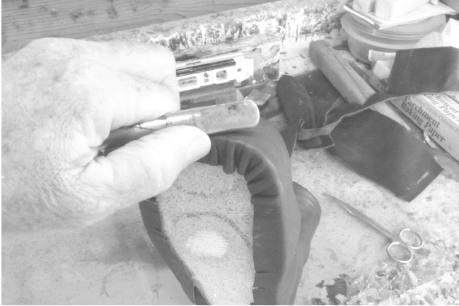
89 The bottom edge of leather is smoothed and pressed as needed to make the corner bottom edge as perfect as possible.
