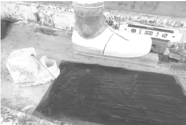
67 The glue for the leather is applied twice, the glue for the area to be leathered on boot is applied once.
