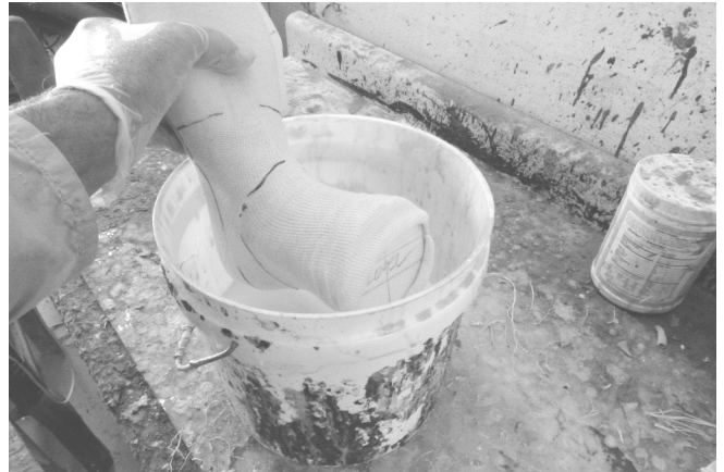
12 The socked boot is dipped in latex with a 40 to 60 percent solids to water ratio.
