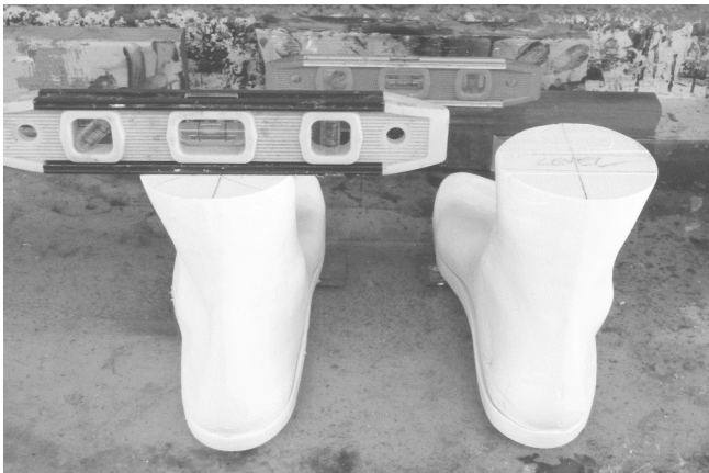
1 The preliminary work has been done. The cast has been prepped. The last has been finished, inserts made and attached. The levelness of stance has been set for a natural vertical or medial/lateral tilt for each last.
