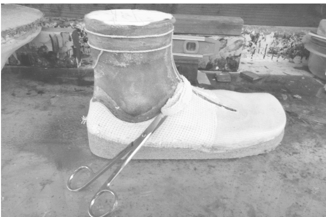
51 Trimming away excess Monks Cloth and sock at design cord. This pair of boots will have soft uppers above the design cord (no Monks Cloth or sock).
