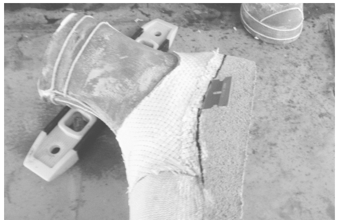
52 Cutting off unwanted bottom Monks Cloth with a razor blade.
