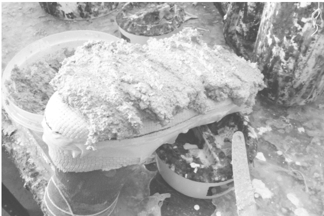
25 The "mud" is applied to an upside down boot.
