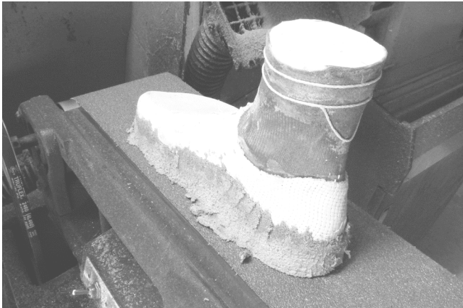
35 The bottom is sanded flat on a flat belt sander.
