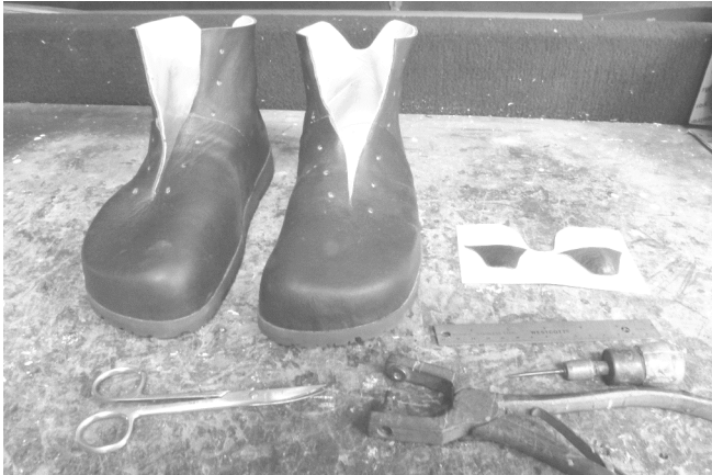
119 The eyelet holes are marked and punched.
