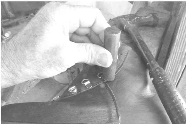
121 The rivets are set with a steel and hammer.
