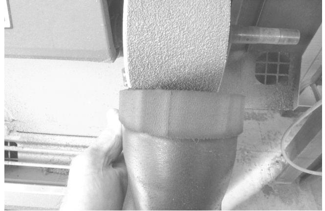
102 The bottom of soling is rough sanded to make the desired thickness and taper from ball to heel and ball to toe.
