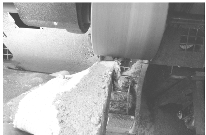
34 After another 12 to 24 hours of drying, the rough sanding begins to remove any unwanted but dry "mud". Stop sanding before you enter the soft "mud" which is not dry.
