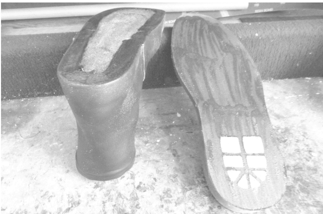
97 The mid soling and heel wedge material are glued (2040 Vibram®). Notice the heel void has been filled with "mud" and sanded flat.
