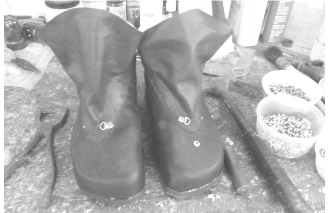
120 The tongue is applied, stitched and speed lace rings and rivets are put into place.
