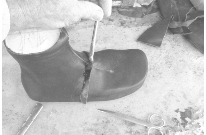
90 Glue is applied to the side seam.
