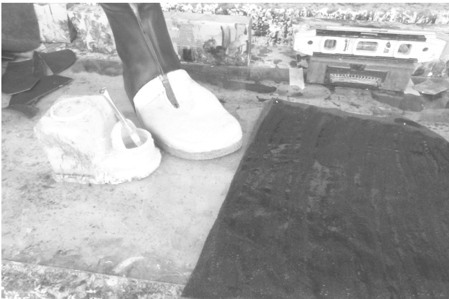
79 Glue is applied to the front leather and front of boot.
