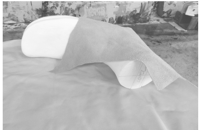
2 The lining leather is measured and cut.
