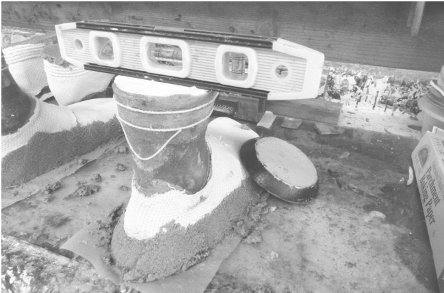
31 The boot may be weighted to help keep the level bubble centered. A fan is turned on and the "mud" is allowed to dry 12 to 24 hours.
