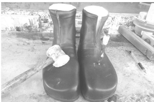
109 The bottom of lace opening is punched.
