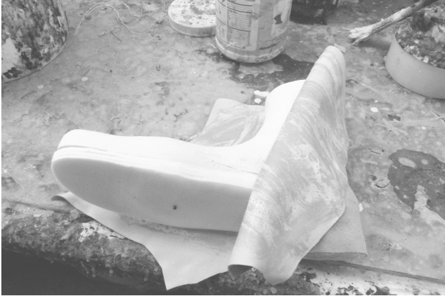
5 The lining leather is pushed, pulled, stretched and pressed onto last until it conforms to the shape of the last.
