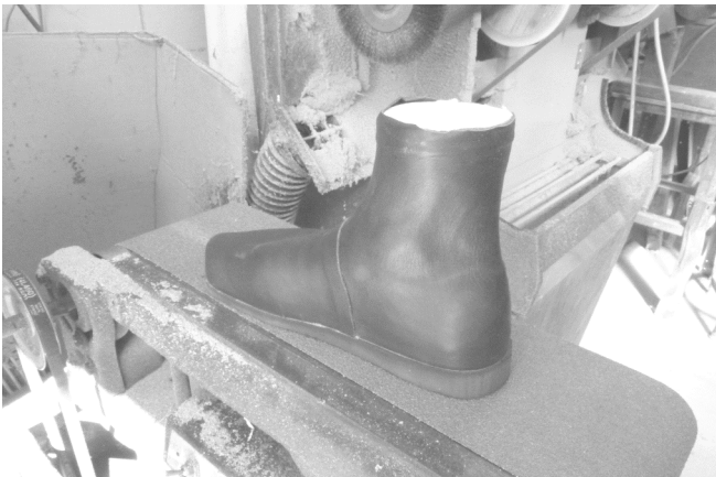
103 The flat belt sander is used to finish the sanding process.
