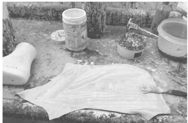
4 The lining leather is latexed with about a 40 to 60 percent solids to water ratio mixture.
