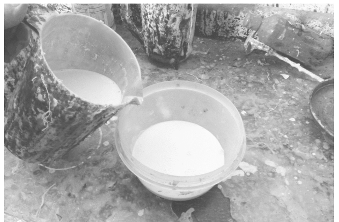
22 The "mudding" latex of about 40 to 60 percent solids to water ration is poured into "mud" mixing bowl.
