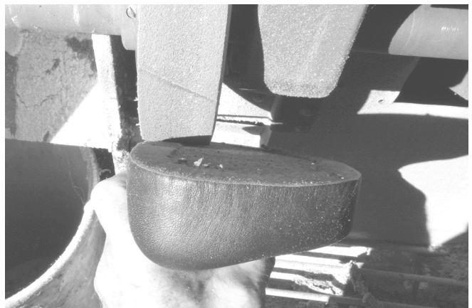
94 The underlap is sanded with emphasis on flatness and a true perpendicular outer edge to bottom angle unless otherwise desired.
