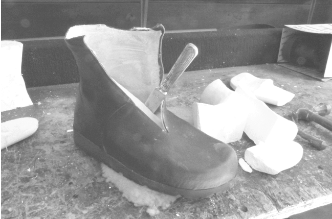
113 The inserts are lifted out with a butter knife.
