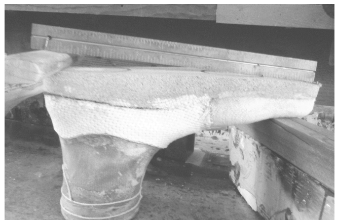
58 The heel lift (heel to ball and ball to toe angles) is checked.
