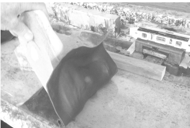
69 The leather is pulled, stretched and pressed on to the boot.
