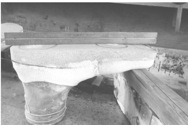
57 The bottom heel to ball flatness is checked.
