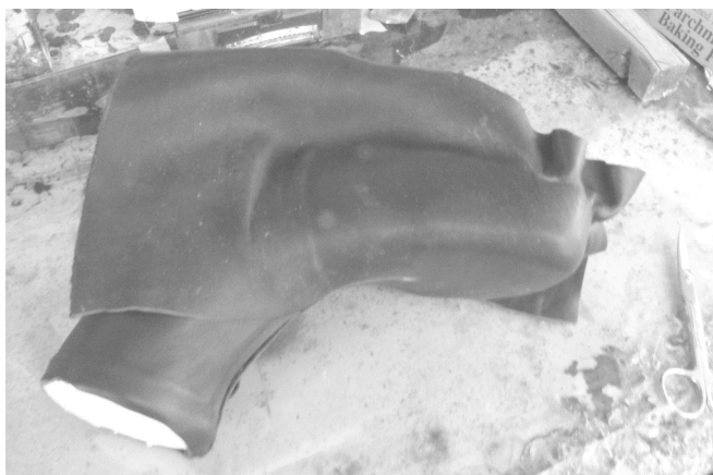
83 The front leather is pressed firmly onto the boot and especially along the bottom edge of "mud".
