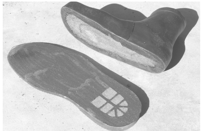
98 After the glue is semi dry and tack free, the sole and boot can be placed in the sun or near a heat lamp for 1-4 minutes. The heat will reactivate the glue and evaporate any remaining solvents. This will strengthen the glue bond.
