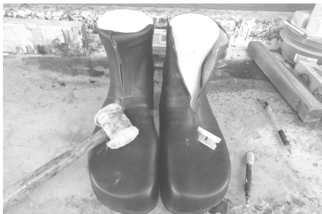
110 The lace opening is cut with a razor blade.
