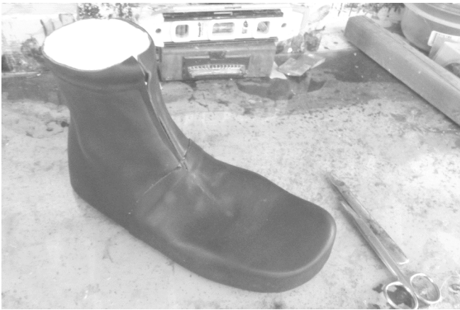
91 The side seam has been bonded.
