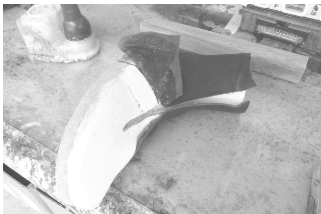
71 The leather at side seam is rolled back to marking.
