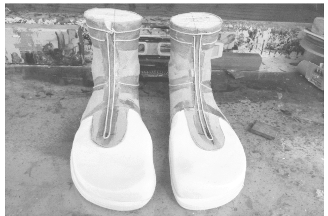
10 The design cords are matched so both right boot and left boot will look like a matched pair. Because of sensitivity of union joints, the bottom of lace opening is offset laterally on each boot.
