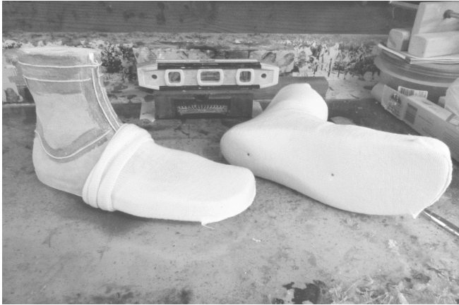
11 Double knit socks are put over last and lining leather. After the socks are on, tacks are located and lifted through the socks. Markings can be put on socks to locate desired positions of Monks Cloth edges.
