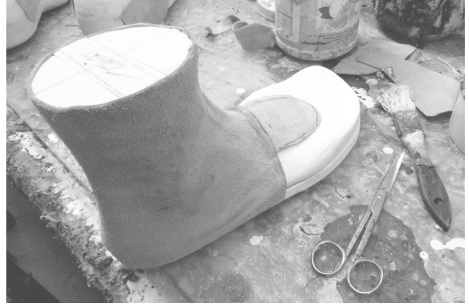
6 This will be a short lining (no lining over toe box area) so a small piece is added under tongue and rivet area.
