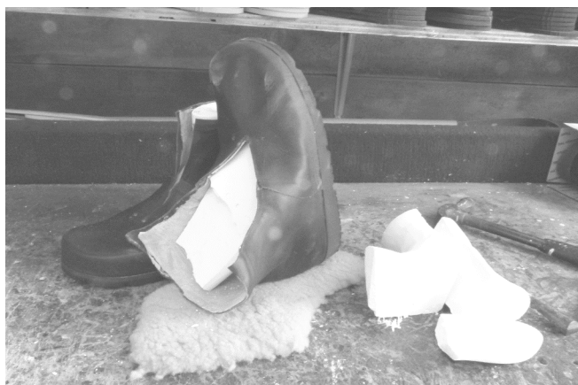
112 The back of the boot is taped against a sheep skin to get the toe part of last to fall out of toe box area.
