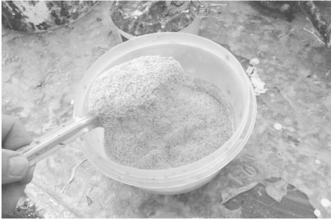
23 A dry mixture of wood flour and cork is put into bowl and mixed with the latex.
