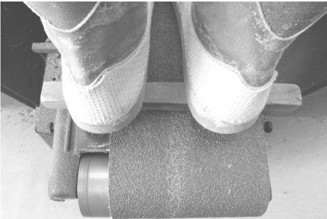
61 The touch up "mud" has been sanded. The fullness and roundness of the outer edge of heel areas are compared for uniformity. They may or may not be a perfect match.
