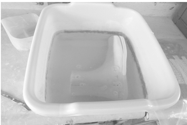
3 The last with inserts is soaked in water one to two minutes.
