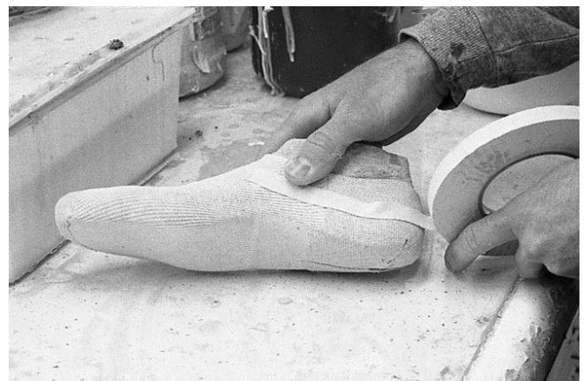
80 Masking tape is applied to dried sock and heel Monks Cloth. The back heel Monks Cloth is used for stiffening. It is referred to as the counter or heel counter in general shoe making.
