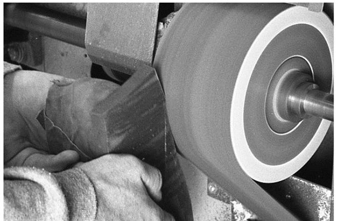
170 The block is cut with a hand knife and then the sides are sanded with coarse grit belt on grinder.
