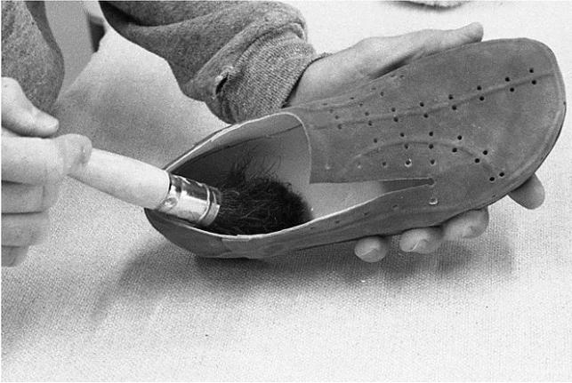
197 Inside of shoe is cleaned again with a hand brush or possibly compressed air.
