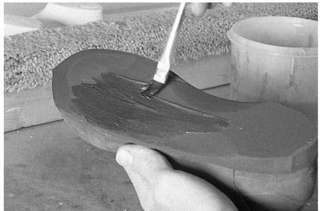
176 Adhesive is applied to bottom of mid soling and wedge.
