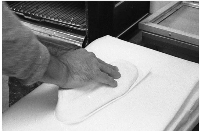
6 The Pe-Lite® is placed on foam. The last is placed on top of the Pe-Lite®. Hand pressure is used to force last into foam.
