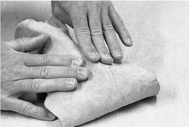
39 Heel lining leather is folded over front leather and is pressed to bond.
