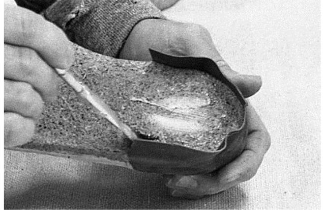
142 Glue is applied to bottom of base inside leather. Then leather is folded to bottom (not shown).
