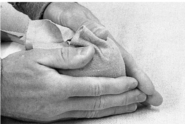
43 Heel lining leather is pressed to insert.
