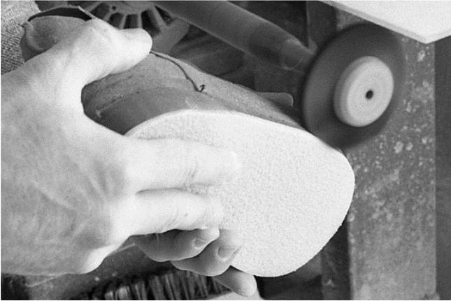
185 Dental lab brush is used to clean leather to sole area and remove burrs and dirt.
