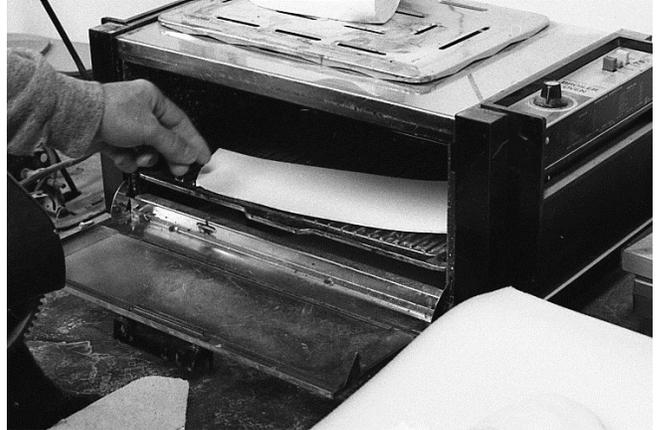
4 The Pe-Lite® is heated for about 30-45 seconds at approximately 250-275F.
