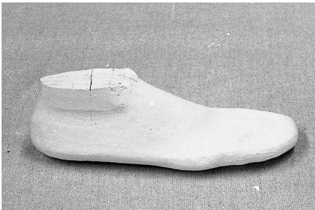
1 Lateral view of foot last ready for shoe construction. The inside form of the finished shoe. The inside SPACE for the foot when the shoe is completed.
