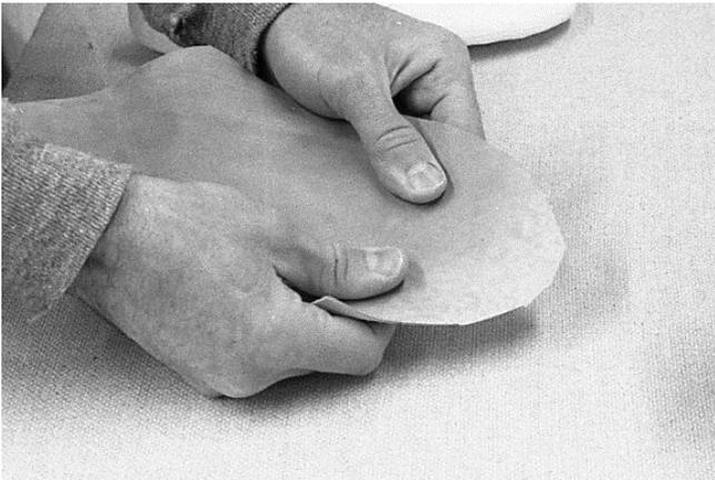
17 The leather is pressed into Pe-Lite® and any wrinkles in leather or bubbles are smoothed and pressed out.
