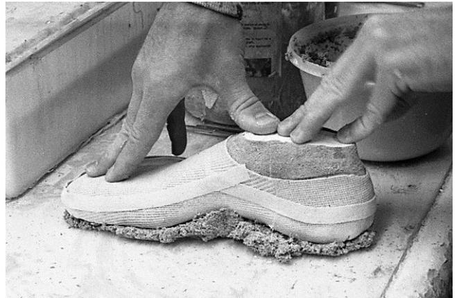
90 Last is flipped and pressed onto glass surface.
