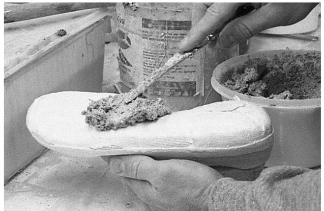
86 "Mud" the mix of latex, wood flour and cork, is applied to bottom of socked last.
