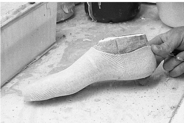
79 Ditto. Sock is now left to dry. The drying takes about a day. It can be speeded up with a fan or heat.
