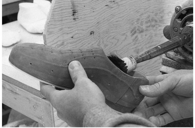
196 Inside of shoe is cleaned with a toe brush.
