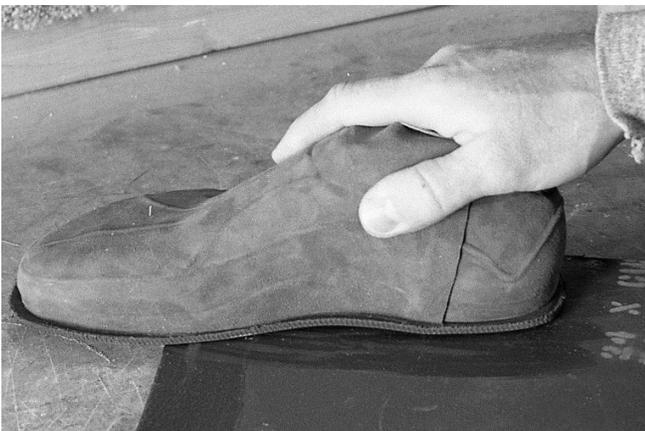
169 After adhesive dries tack free, the shoe is placed on cushion block, from ball to heel.
