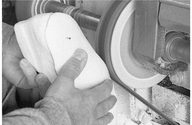
24 Edge of insert is sanded smooth right up to the last for a really nice and close fit.
