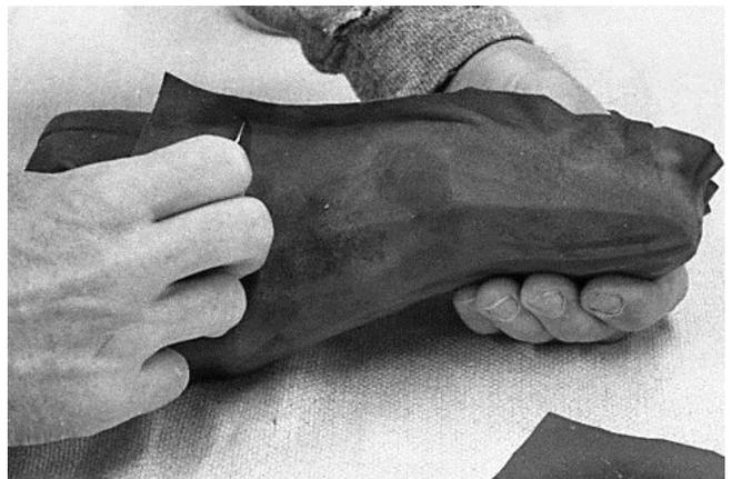
152 Front leather is pressed with blunt (not sharp) tool just in front of overlap. The overlap is 1/4" to 3/8".
