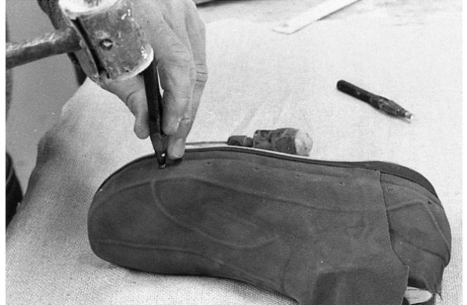
186 Base perforations are punched with a #3 punch.
