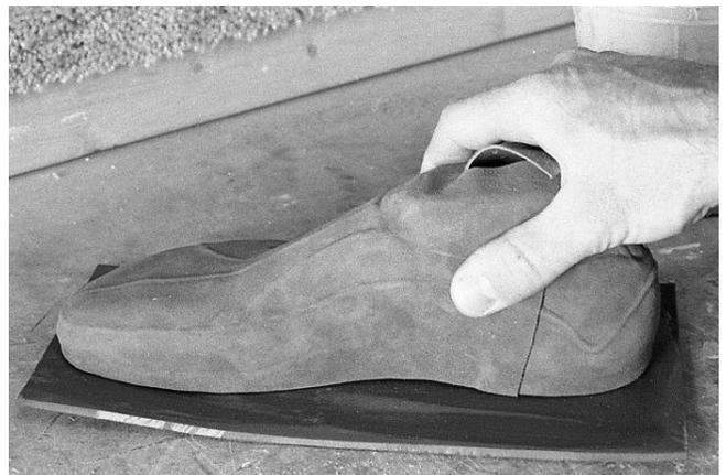
164 After adhesive dries tack free, the shoe is pressed into mid soling and hand firmed so there are no voids in the bond, especially at edges.
