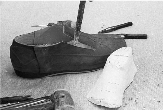
191 Last is removed from shoe with care to do as little damage to last as possible, so it can be reused again.
