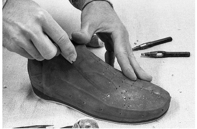
190 Single edge razor blade is used to cut lace opening from bottom hole upwards.
