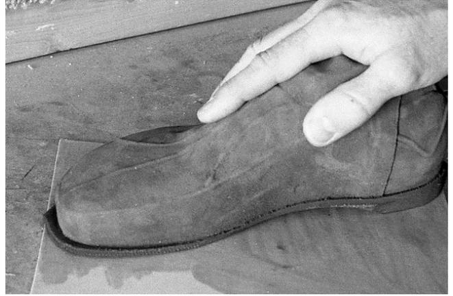
178 After being allowed to dry tack free, the shoe and outer sole are pressed together.
