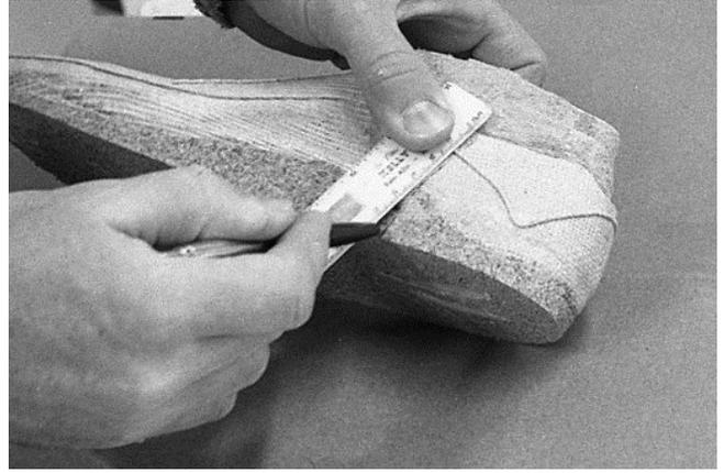
130 Marking medial front edge of heel seam.
