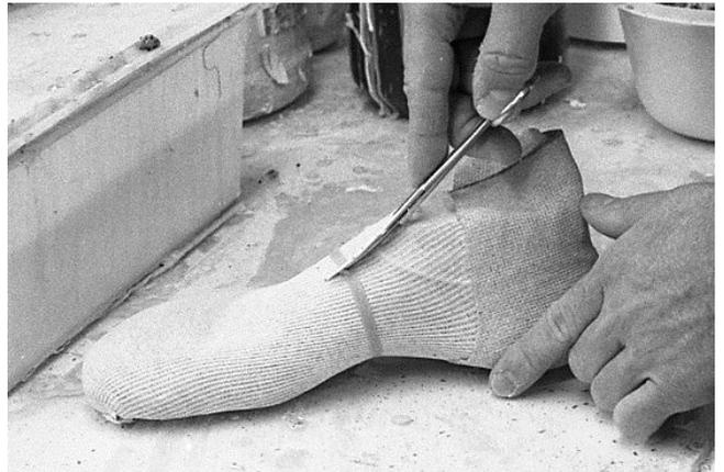
72 Sometimes a rubber band can be used to force latexed sock to hold to last temporarily while latex sets or firms.
