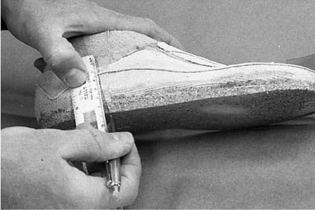
129 Marking lateral front edge of heel seam.
