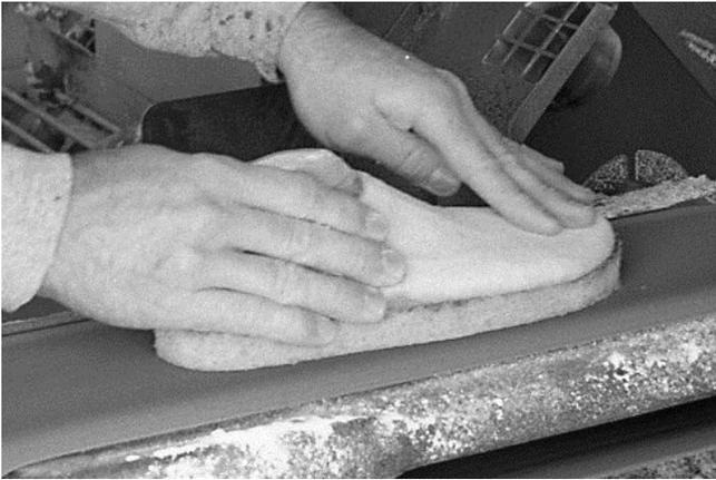
101 A flat bed belt sander, running away from the artisan, is used to grind the flat bottom surface.
